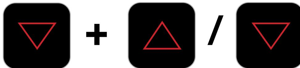
*On 2U Imperium only:* Hold Downwards pointing Input arrow, then toggle Level Arrows up or down to either **increase or decrease display intensity**
